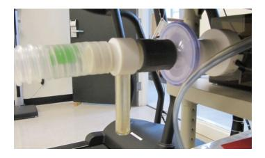
• The result will be something like this. The weak point is the hose mating with the T-connector. Ensure a good connection. If this separates during testing, continue testing and re-attach as quickly as possible
