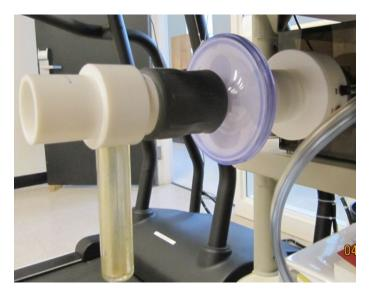
• The hose can be attached to the reticulated arm using Velcro straps. The black device (with the orange dot) is the heart rate monitor receiver (the chest strap on the subject is the transmitter). Take the far end (from the cart) and attach to the T-connector/pneumotach assembly. Ensure the hose is parallel to the floor.
