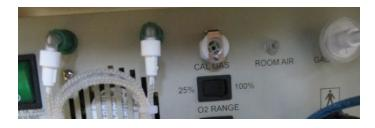
• This is what you want to see. This connection can be left intact up to and including testing. Remove when you are finished. Turn off the calibration gas cylinder by turning clockwise hand tight. Then bleed of the excess left in the regulator and the calibration gas hose/white connector by gently pushing on the plastic connector/opening at the end. Bleed off until both indicators read zero
