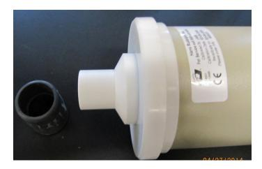
Attach the grey connector to the syringe
